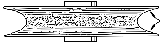
PULLEY NOT ALIGNED CORRECTLY
